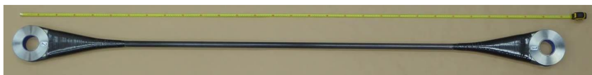
Figure 1. CFRP tendon of 2730 mm length and 33 mm diameter with titanium thimble (cable eye)
