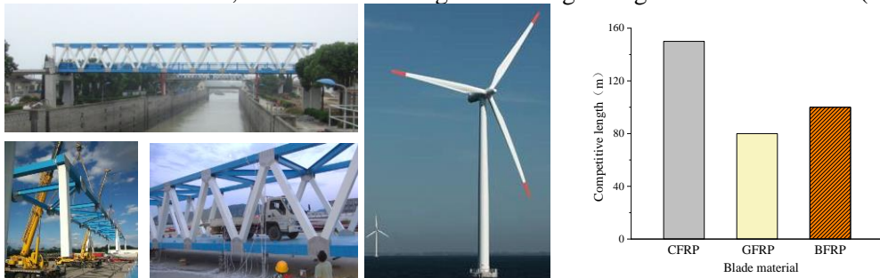
Figure 7 Long-span BFRP truss structures and ultra-large-radius wind turbine blade
